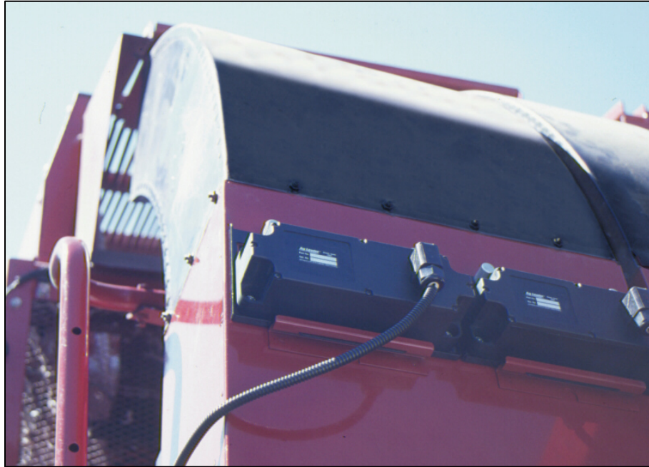
Figure 1. Optical AgLeader Mass Flow Sensors on Air Duct
