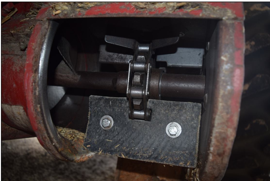
Figure 11. Clean Grain Elevator – Chain and Paddle Case IH Combine
